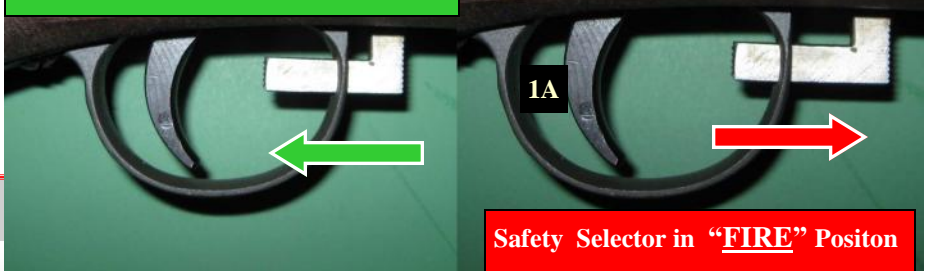
Safety Selector in “ SAFE ” Position
